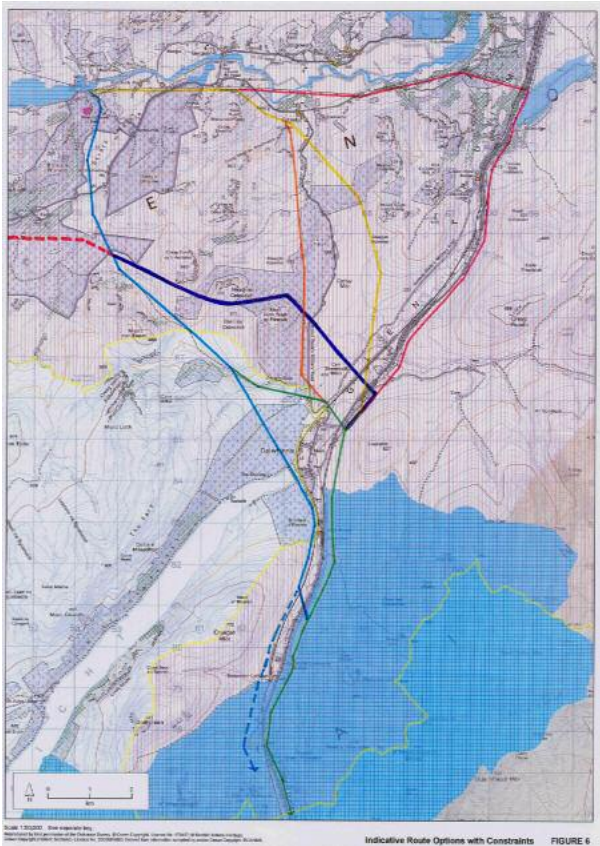
Figure 1: Map showing original route options, with link to new route shown dashed-red; from there the new dark blue route takes the line further north from Dalwhinnie, joining onto the green line which then follows the eastern side of the A9 south. (Park boundary shown pale-yellow).
